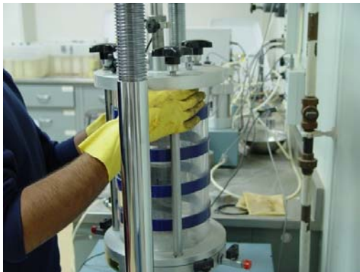
Placing the triaxial cell
